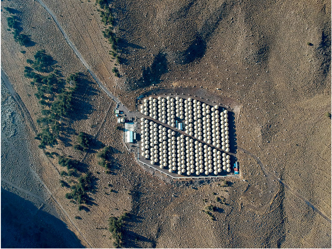
Figure 2.4: An aerial shot of the HAWC array. The large tanks are the main array while the smaller tanks are part of the outrigger array. The off-center building at the array's core is the counting house. The outriggers are currently not considered for data collection. Photo courtesy of Dr. Jordan Goodman of the HAWC collaboration.
