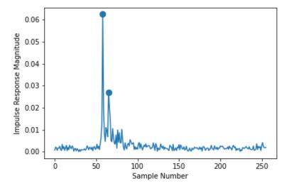
**Figure 1.** An example of feature extraction from the KWAUG14 channel impulse response. Significant arrivals have a marker.
