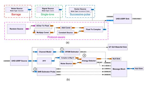
FIGURE 3. Simplified GNURadio flow graph for (a) launching the jamming attacks and (b) extracting the radiometric features.
