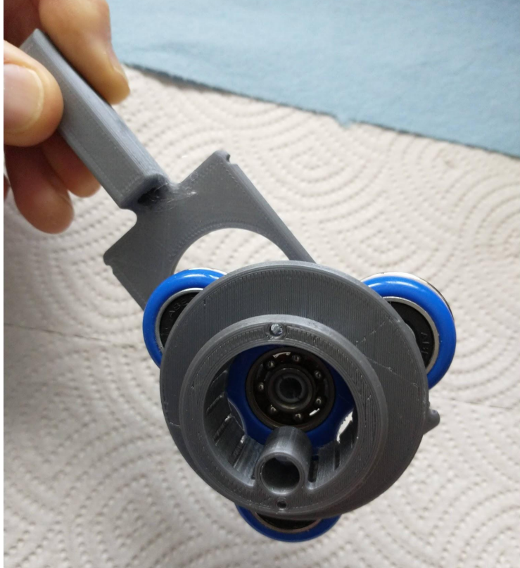
Here are the three parts assembled together with the spinner, but without the coil-LED board.
