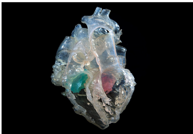
Fig. 4. Model of the heart and major arteries using a polyjet 3D printer.
