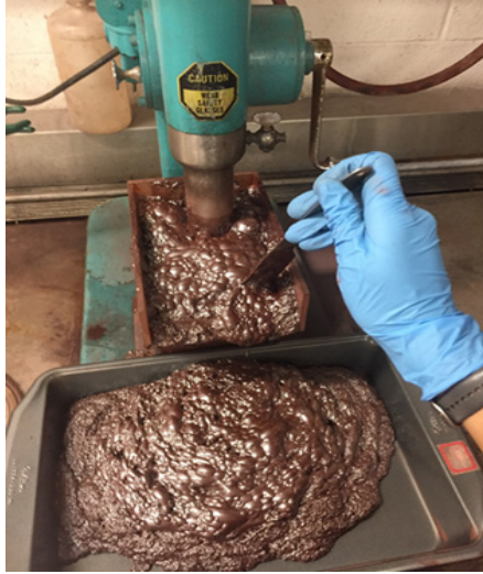
Figure 3.4: Flotation set up in the MTU laboratory. Tailings were recovered in the froth product and the concentrate was recovered at the bottom of the flotation cell.
