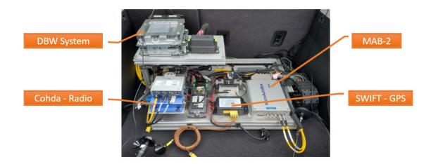
Figure 5 Vehicle Instrumentation in boot
