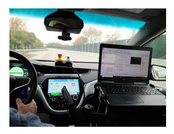
Figure 6 Laptop connected to vehicle performing real-time vehicular control.
