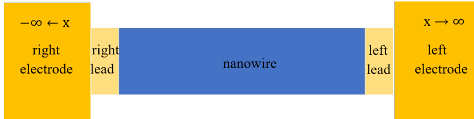
Figure 3.1: A schematic showing a two terminal nanowire junction; the nanowire together with the leads form an active scattering region.
