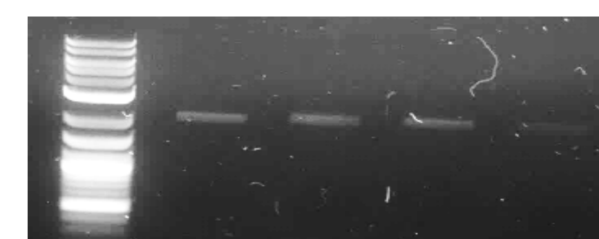
Figure 3. Insert Post-PCR, Digestion, and Purification. Lane 1: 1kb NEB ladder, Lane 2-5: Multiple prepared inserts.
