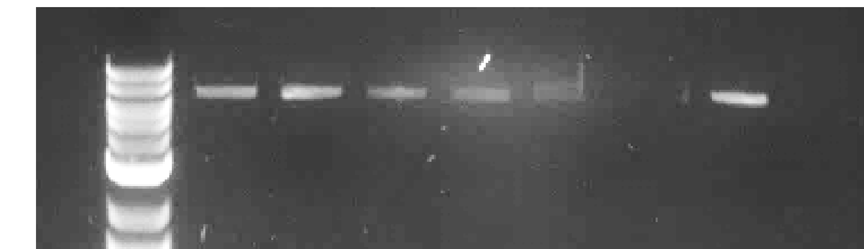
Figure 5. Vector Post-Digestion and Purification. Lane 1: 1kb NEB ladder, Lane 2-9: Colony 1-8 miniprep, digestion, and purification products. Colonies 1-5, and 7 were utilized in subsequent steps.
