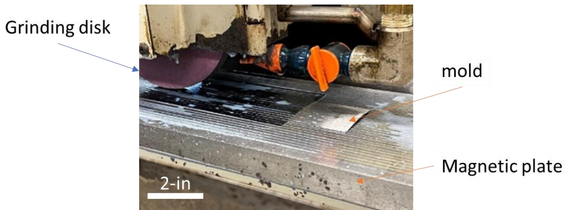
Figure 74. Photo of A003 On surface grinding machine
