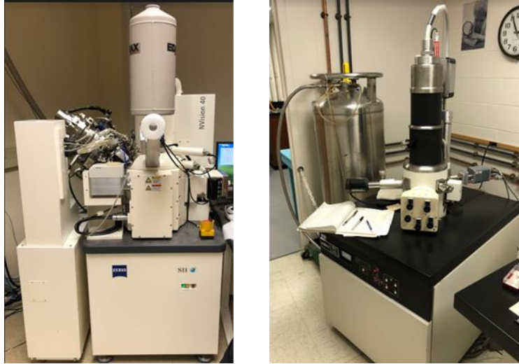
Figure 47. SEM machines: Nvision 40 (left) and AMRAY 1820 (right).
