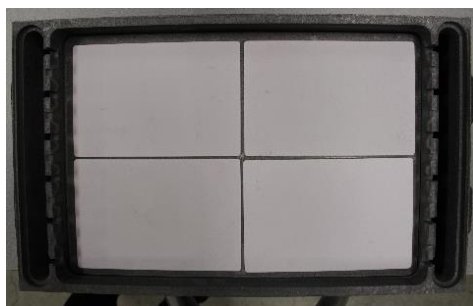
Figure 11. Furnace tray with 4 setter plates
