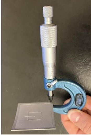
Figure 77. Vernier micrometers with a cone tip placed on the ablated surface (shown) and a flat anvil on the non-ablated surface (not shown) measuring the thickness of A003.
