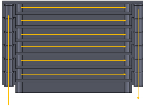
Figure 12. Gas flow in the graphite retort
