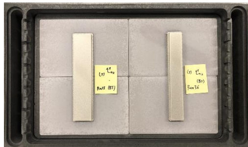
Figure 33. Layout of parts on setters in a retort layer
