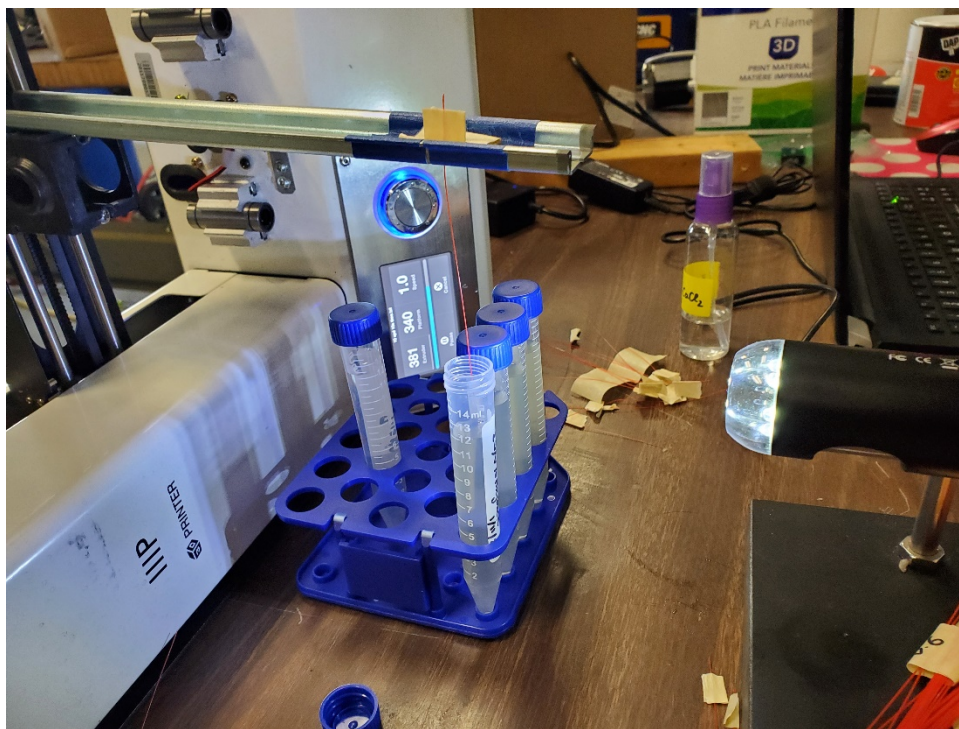
Figure 3.1: The original setup which used the 3D printer axis consisted of a roughly attached metal bracket. A slot in the bracket was covered with tape to create a slit for the PLA fiber to pass through. Masking tape was added to the upper end of the fiber to allow it to hang from the bracket arm.
