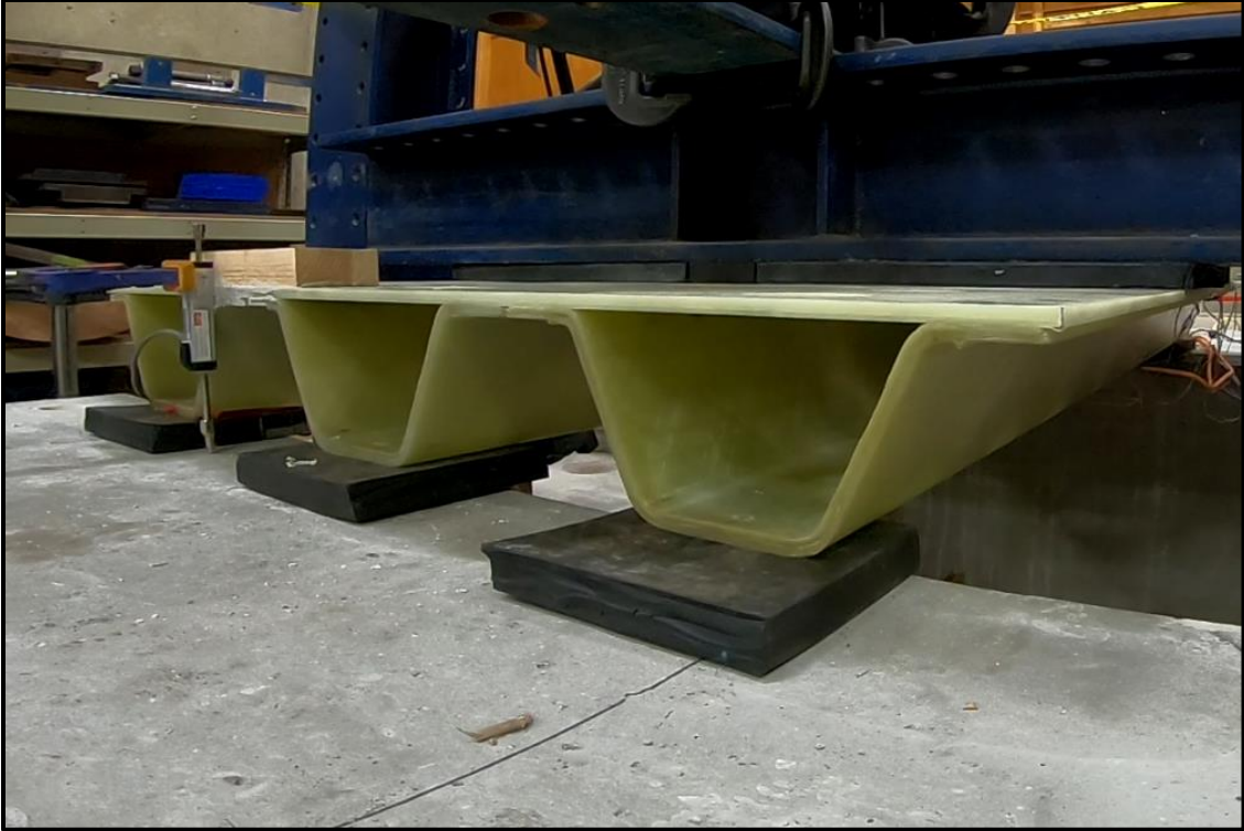
Figure 92: Photo before Testing of Panel 1 – No Load
