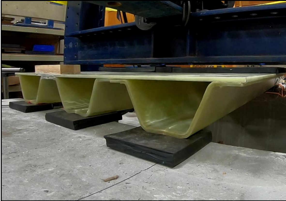
Figure 94: Photo after Testing of Panel 1 – No Load
