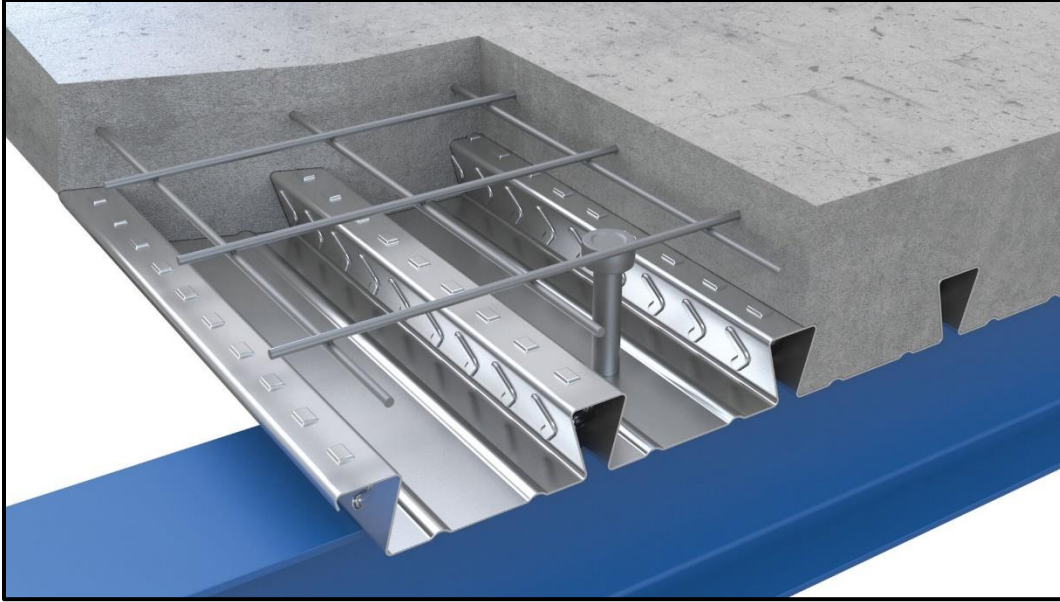
Figure 2: Stay-in-Place Steel Formwork [2]
