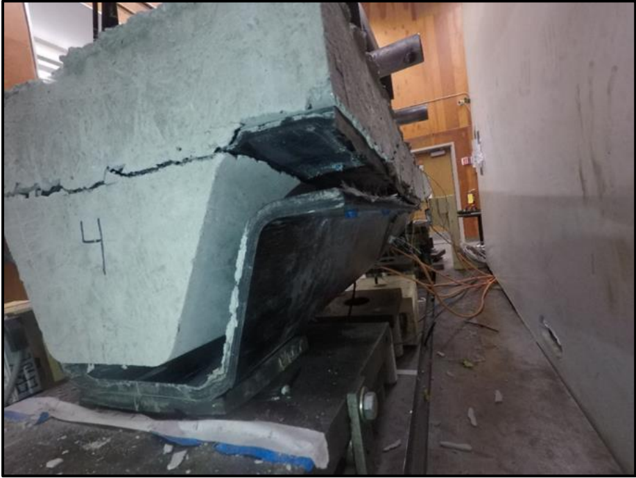
Figure 35: Failure of Specimen 4 – End and Side View
