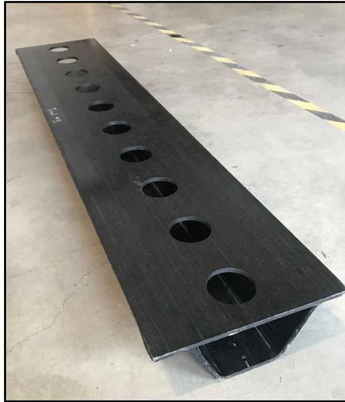
Figure 25: Completed Closed-Corrugation Part
