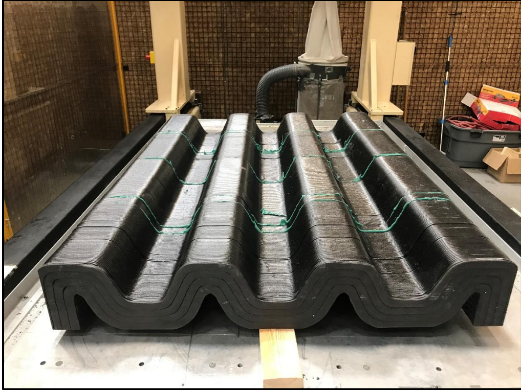
Figure 76: 3D Printed Mold Ready for Machining
