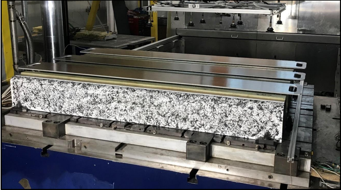
Figure 80: Corrugation Prepared for Secondary Bonding with Spring Table
