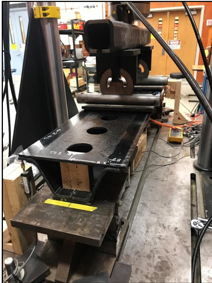
Figure 29: Test Setup for Single Closed-Corrugation Specimen
