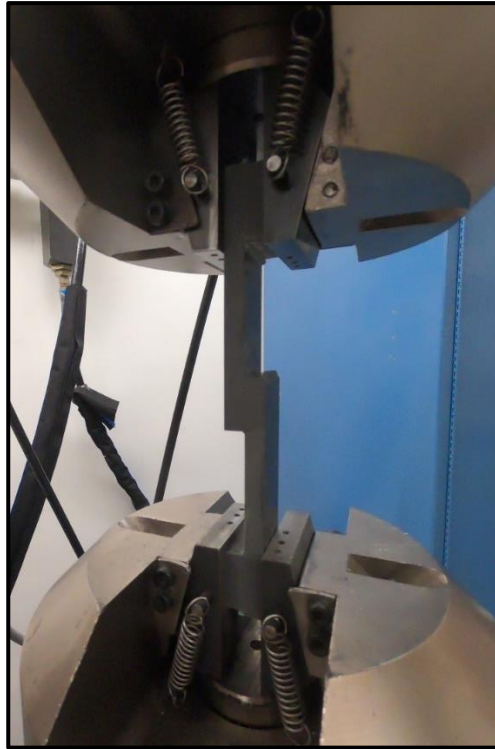
Figure 51: Lap Shear Coupon Loading into Instron Machine
