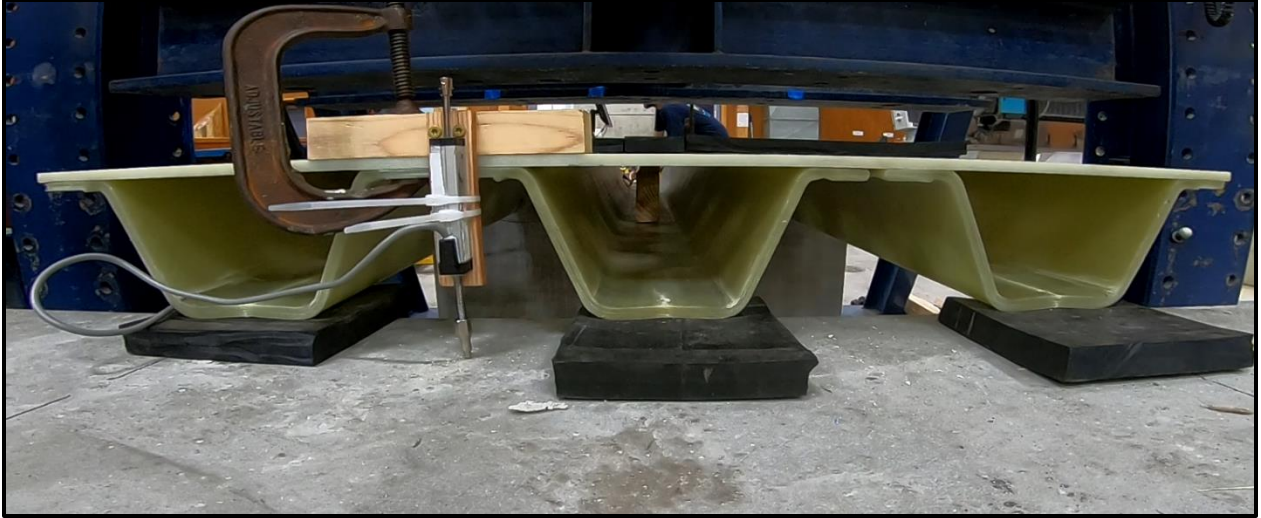
Figure 95: End Cross Section View after Testing of Panel 3
