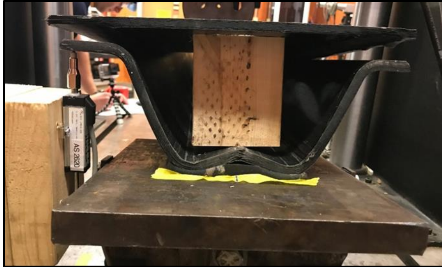
Figure 33: Failure of Specimen 1 – End Cross Section
