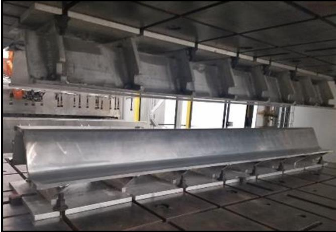
Figure 20: Stamp Forming Mold Positioned in the Press
