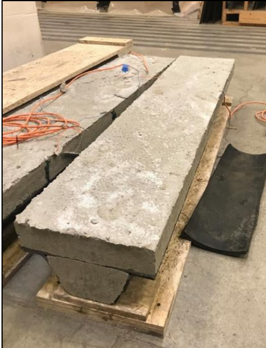
Figure 27: Completed Hybrid Closed-Corrugation Specimen
