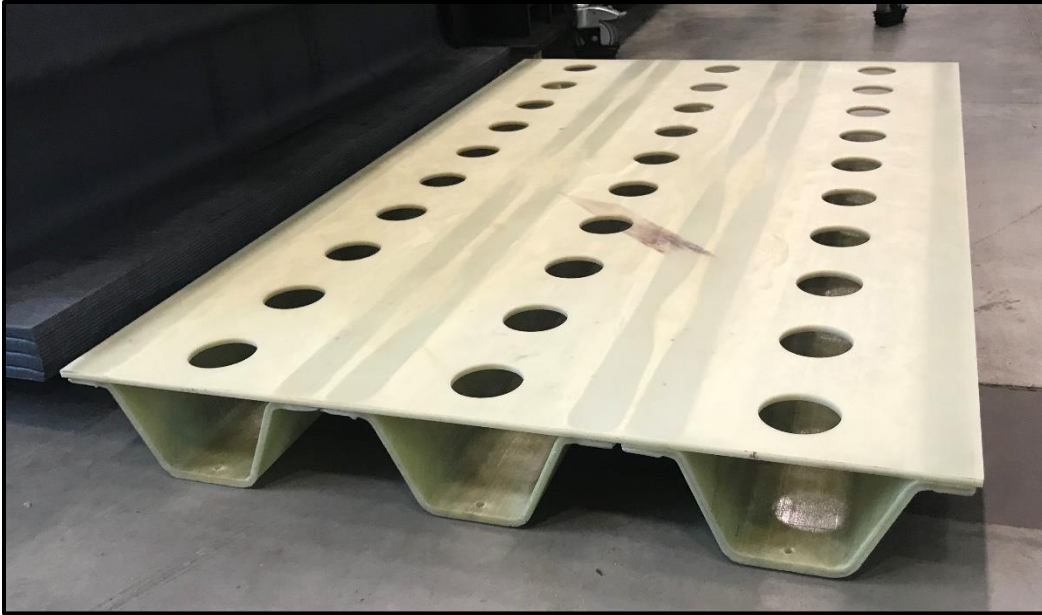
Figure 81: Completed Multi-Corrugation Panel
