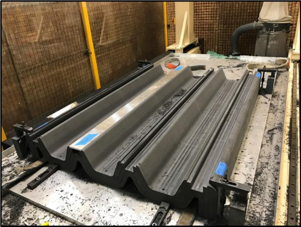
Figure 78: Fully Machined 3D Printed Mold
