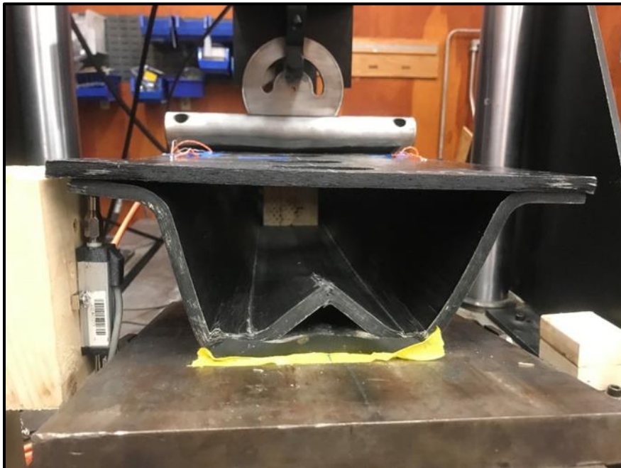
Figure 34: Failure of Specimen 2 – End Cross Section
