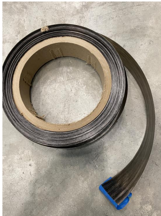
Figure 3: 50 mm wide CFRTP composite tape
