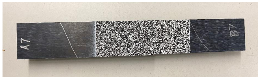
Figure 12: Typical bearing specimen with painted DIC pattern
