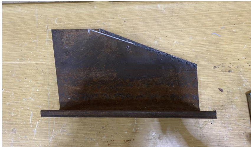
Figure 35: Steel replacement for truncated hinge
