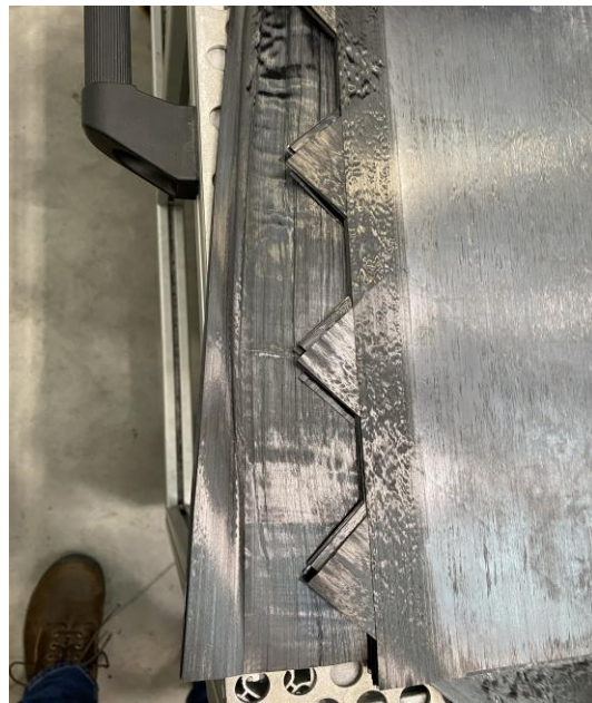
Figure 38: Flange fiber squeeze out
