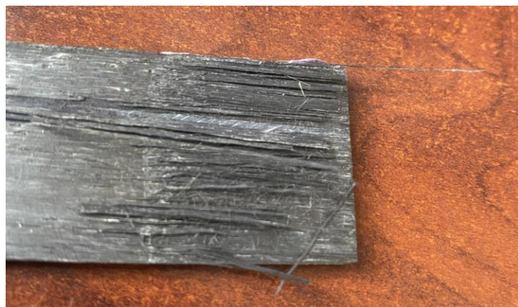
Figure 22: Failed Adhesive 2 Specimen
