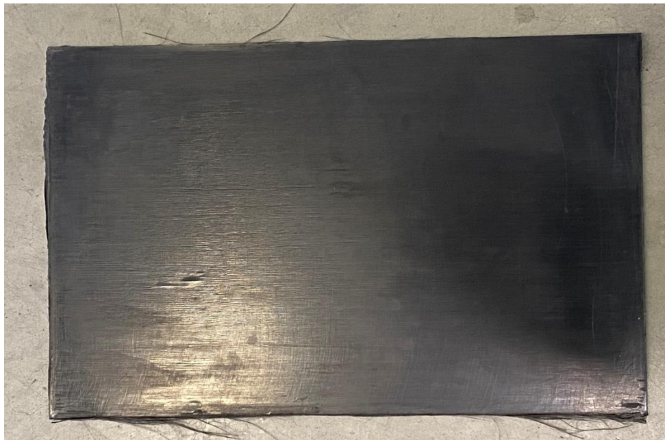
Figure 10: Consolidated CF/PPS plate
