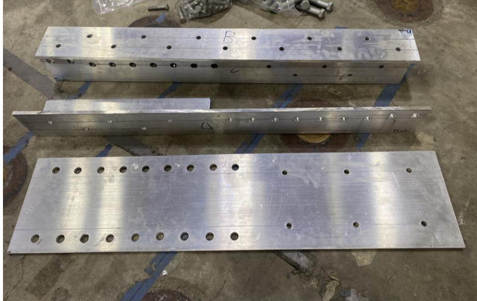
Figure 40: Processed aluminum members
