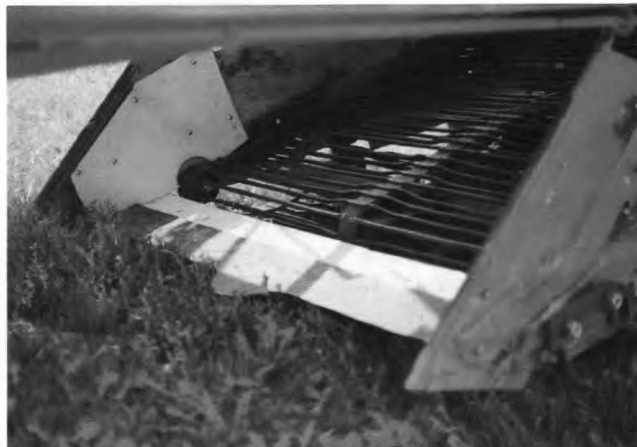
Figure 3: Modified digging spade and primary bed on Aroostook Farm potato harvester.
