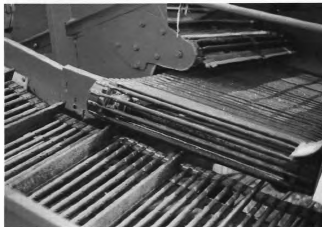
Figure 4: Modified secondary and rear cross beds on Aroostook Farm potato harvester.
