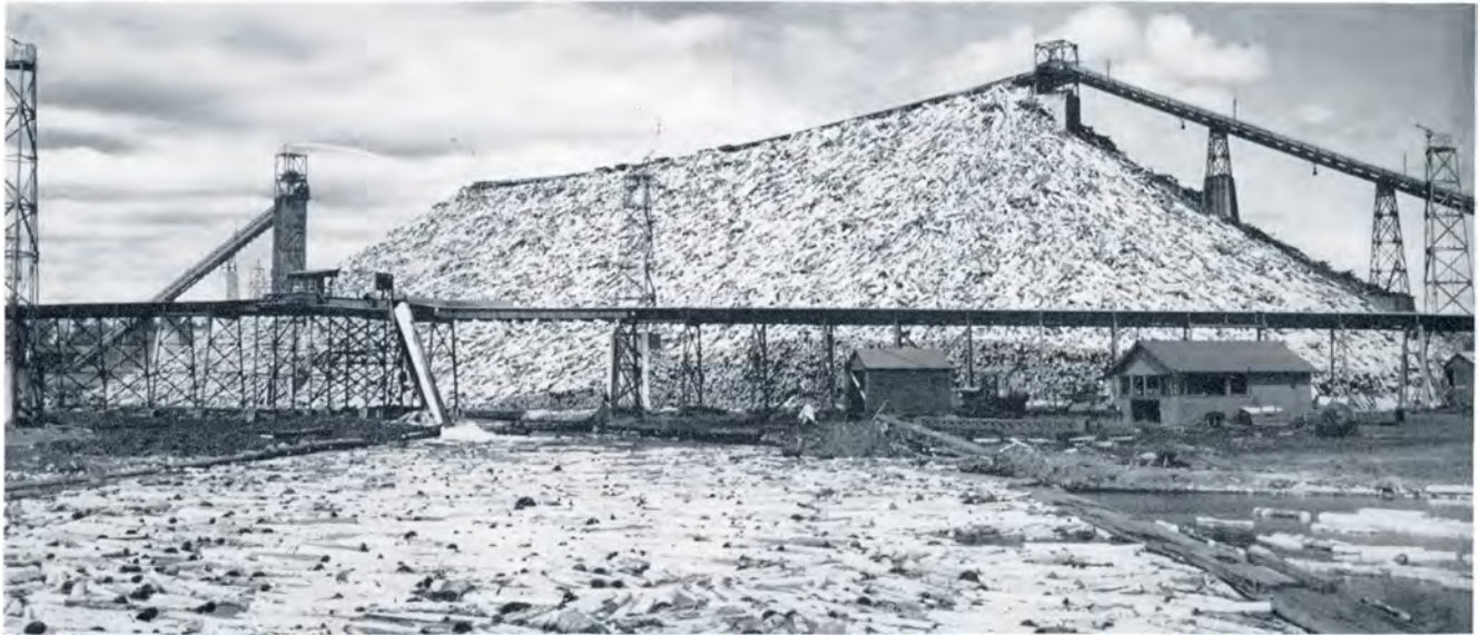
Winter pulpwood storage at Millinocket. Since wood cannot be moved by water in winter, the mill accumulates large piles of barked wood during the late summer and fall for winter use. This pile is about 90 feet high and contains nearly 40,000 cords.
