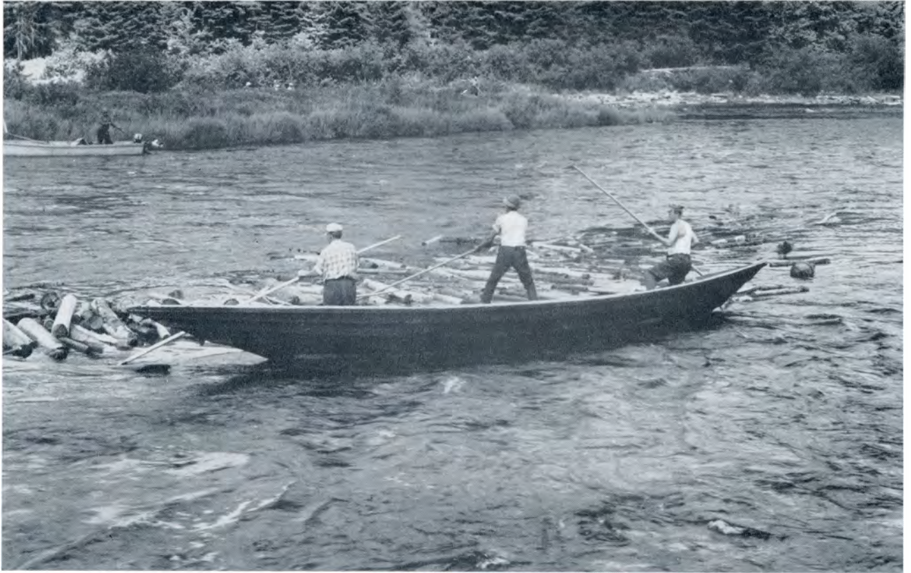
River drivers do a large part of their work from the bateau, which is handled with oars or a pole. For many years, this flat-bottomed, safe boat has been their mainstay, permitting them to reach wood that is stranded on ledges or sand-bars.
