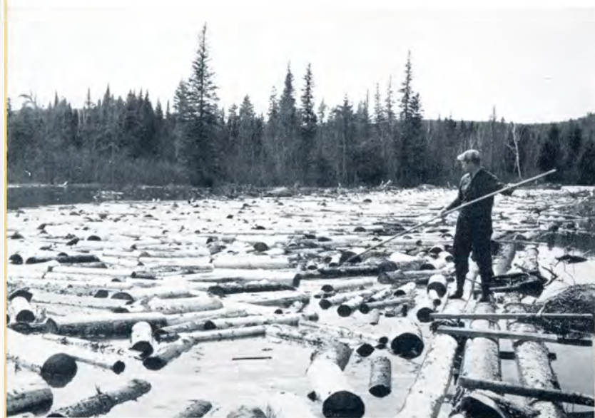
River man poling wood through a sluicing boom to the gate of a driving dam.
