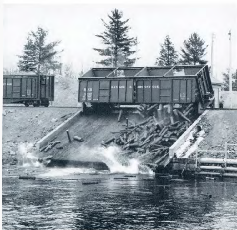
(Above) Special pulpwood cars can be dumped through the swinging side in five minutes. These cars, and the hydraulic tilting device, were designed jointly by the engineers of Great Northern and the Bangor and Aroostook Railroad.
