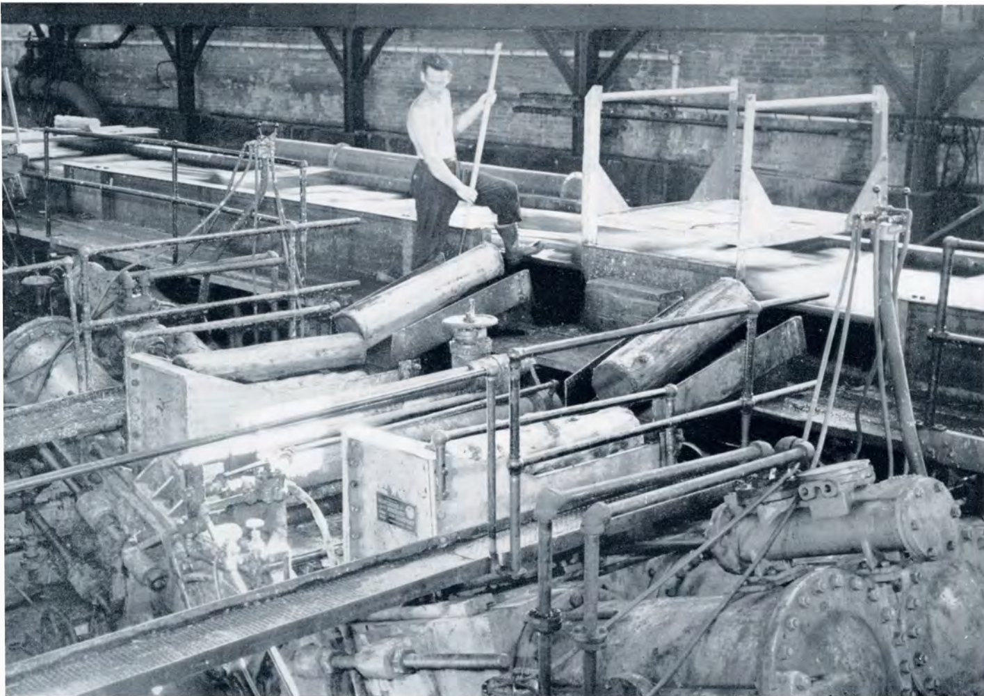
Charging one of the 30 Great Northern pulp grinders at the Millinocket Mill. Each of these machines requires 1,800 horsepower and is capable of producing nearly 30 tons of groundwood pulp per day. This type of grinder was developed by Great Northern and is widely used in the industry.
