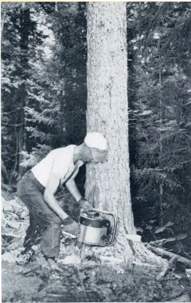
First operation in making newsprint. Power saws, such as the chain saw used by this woodsman have practically replaced the hand saw in the woods.
