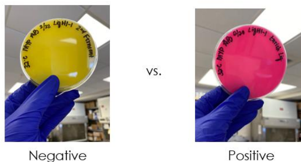
Figure 2.1. Mannitol Yolk Polymyxin (MYP) agar plates comparing negative and positive growth for B. cereus .
