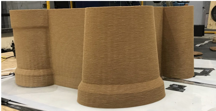
Figure 52: Final printed part with extrusion temperature 207°C and layer time 285s.
