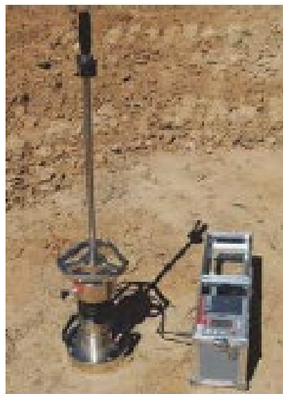
Figure 5.3 Zorn Lightweight Deflectometer with Attached Data Logger (Berney et al. 2013)
