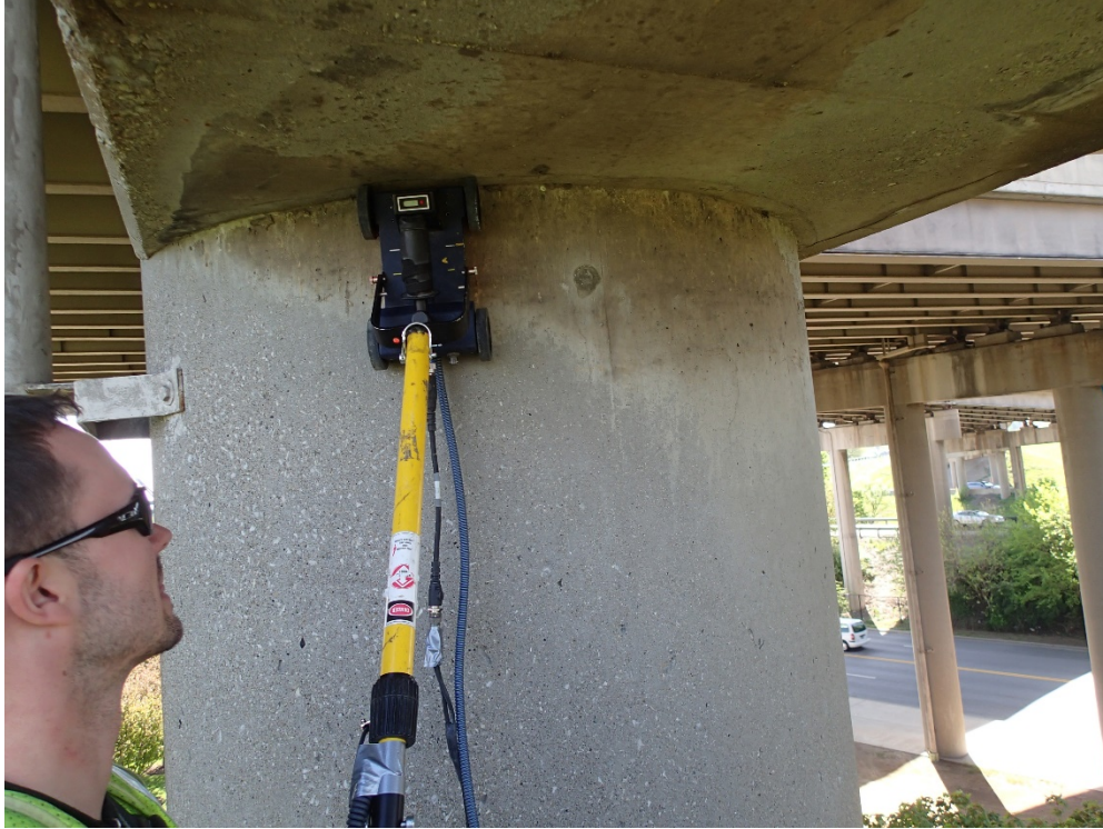
Figure 7 Ground penetrating radar being used to inspect for delaminations on I-65 pier columns (2013)
