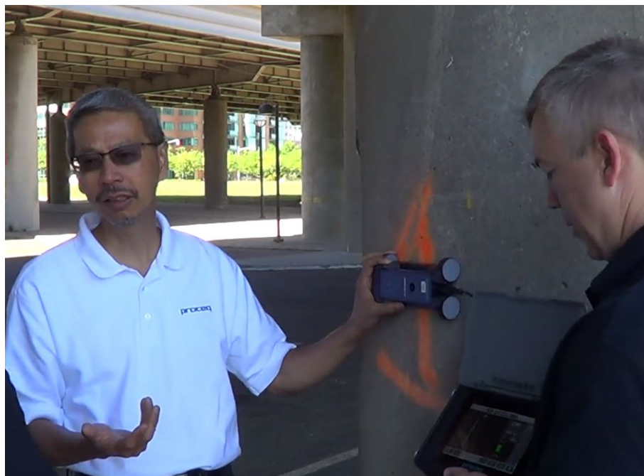
Figure 31 Detecting reinforcing steel and measuring cover depth using a covermeter. The inspector (left) has placed the probe is placed on the column and the measuring unit is being held by the person on the right.
