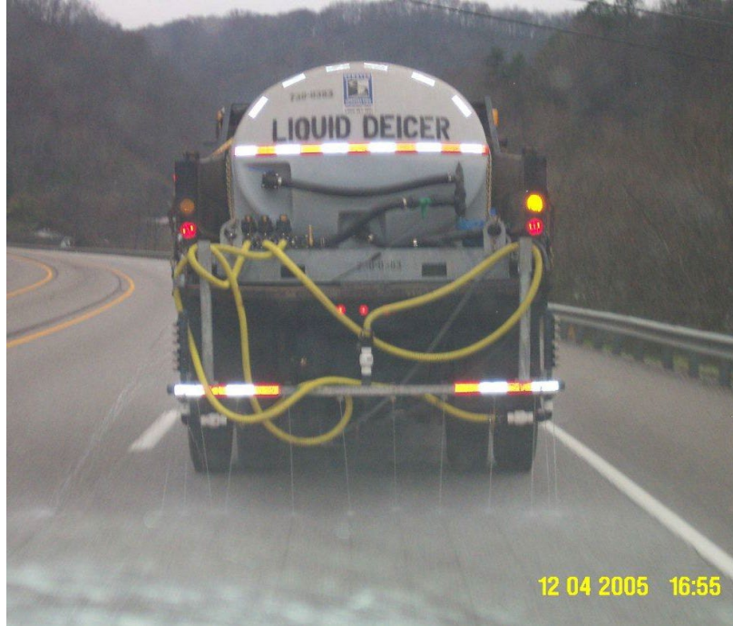
Figure 1 Tank truck applying liquid deicing chemicals to roadway as a pre-treatment
