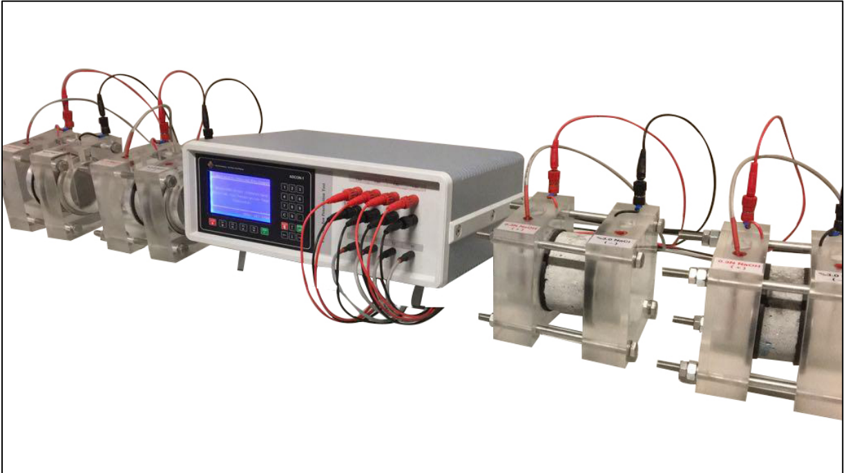
Figure 36 Test apparatus for AASHTO T 277 rapid permeability test (Courtesy Geotechnical Test Equipment Ltd.)
