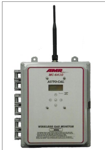
Figure 4.2 Wireless Multi-Gas Monitor (AMR PEMCO, 2002)
