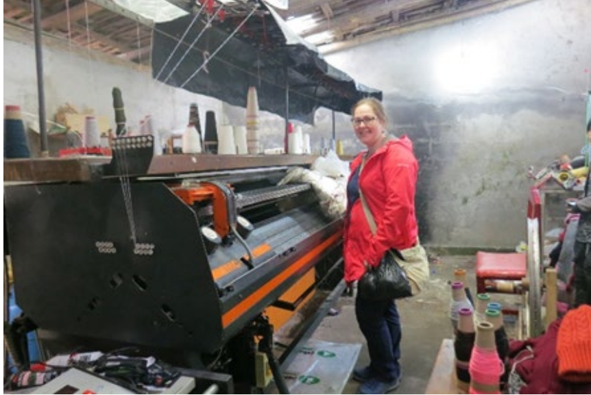
Figure 1.6 Machinated hand weaving is operated either via computer programs (bottom left corner) or cylinders with holes (See Figure 1.5). Once a design has been programmed into the computer, the weaver presses the button, and the machinated loom creates the design. These machines are the most expensive weaving technology used in Peguche. Miguel took this photo on my camera in 2017.
