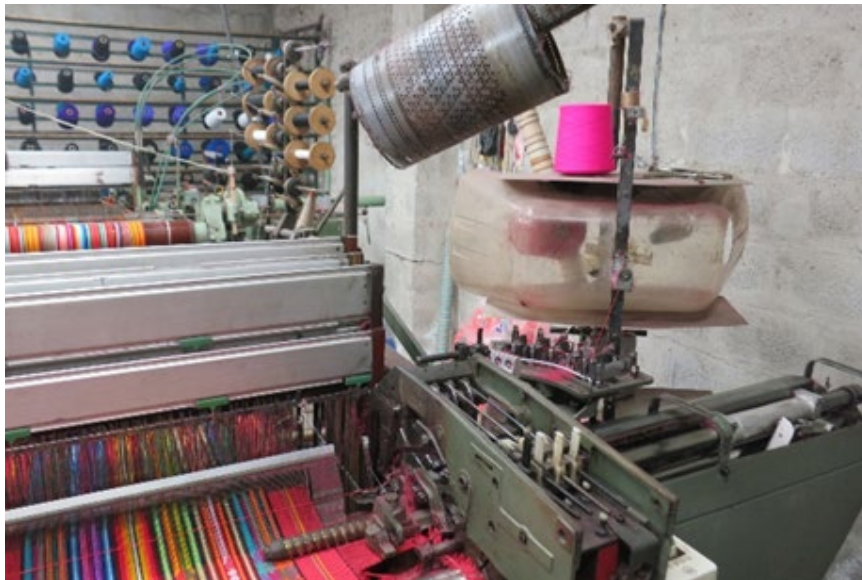
Figure 1.5 Machinated hand weaving is operated either via cylinders with holes (top of photo) or computer programs (See Figure 1.6). The sequence of holes in these cylinders dictates the design that will be woven. [Author photo]
