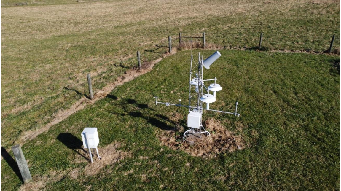
Figure 3.2: The AWOS on the LRC property that collected the atmospheric and soil data.
