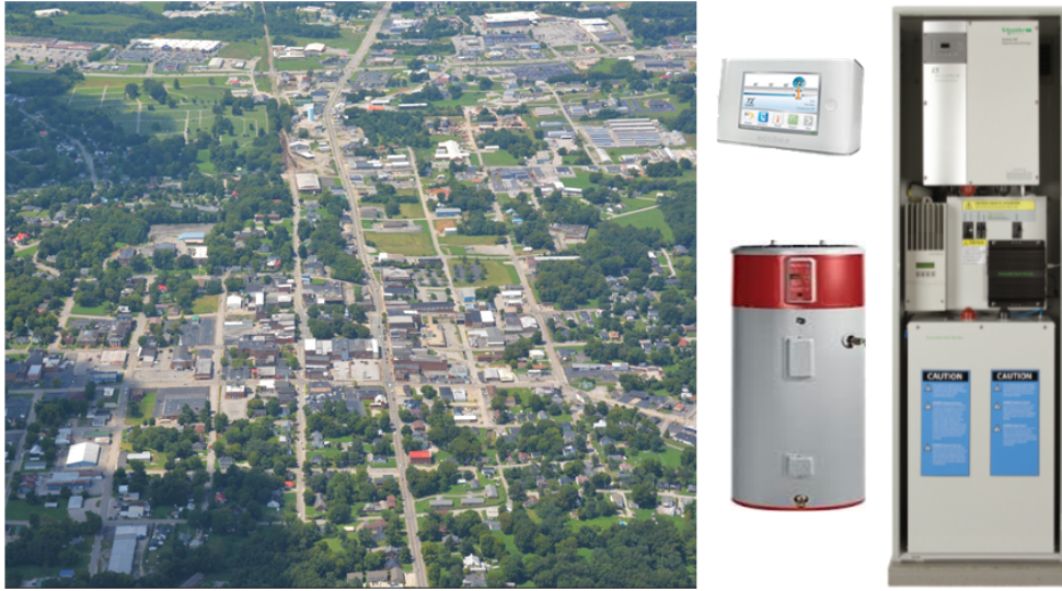
Figure 4.1: Aerial view of Glasgow, KY, the location of the studied SET, along with pictures of smart devices for home energy management: thermostat, EWH and BESS, which are programmable and enabled by WiFi or Ethernet. The data acquired has a resolution of up to 1 minute and is available for both home owners and the utility.
