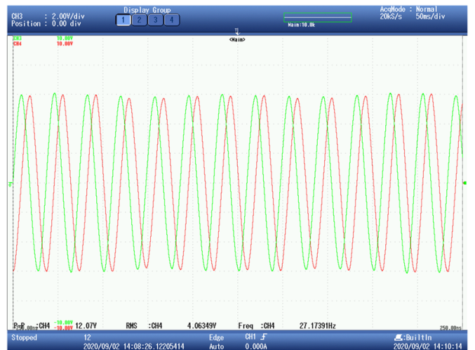
Fig. 11: Measured open-circuit back-EMF at 544r/min for the 2-phase winding configuration. The air-gap length was set to 2.7mm.
