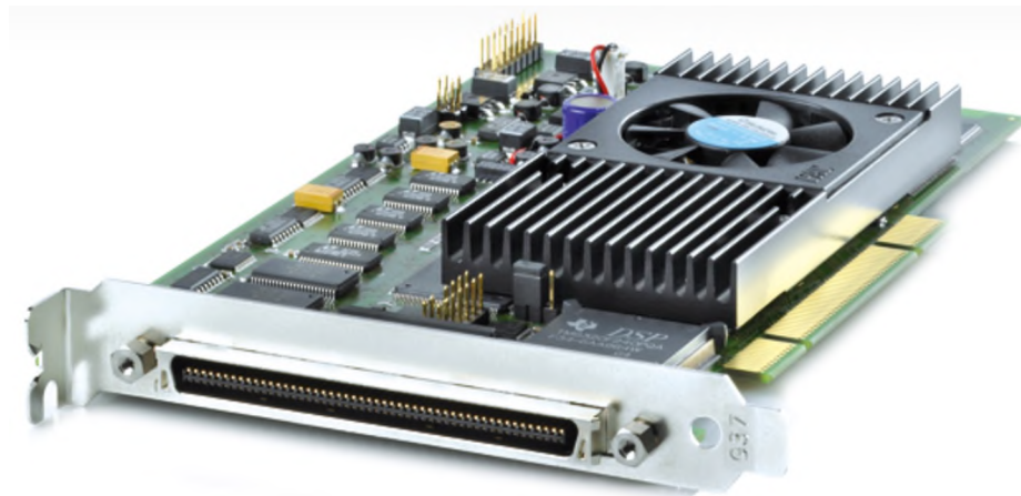
Figure 9: dSPACE DS1104 Controller Board, (dSPACE courtesy).
