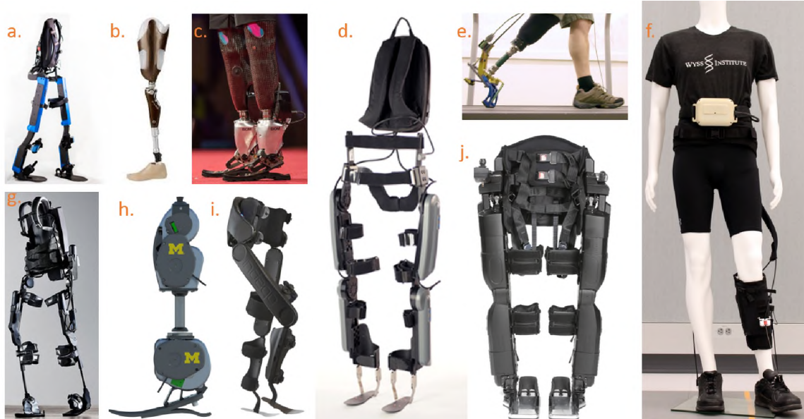
Figure 1: Currently existing powered exoskeletons and P/O devices: a. Mina v2 (ihmc); b. C-Leg (Ottobock); c. Bionic Leg (MIT); d. ReWalk Personal 6.0 (ReWalk) e. Prosthetic Leg (Stanford); f. ReStore™ Soft Exo-Suit (ReWalk); g. PHOENIX Medical Exoskeleton (SuitX); h. Open-source Bionic Leg (UMich); i. Indego (Parker Hannifin); j. REX (RexBionics).
