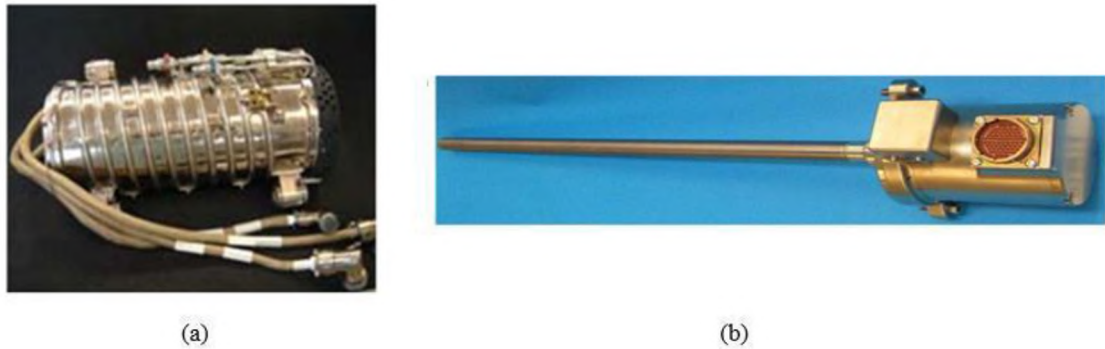
Figure 6. (a) ESA_MSL Low Gradient Furnace (LGF) used for the directional solidification and (b) Sample Cartridge Assembly (SCA), which includes a sample for an ISS directional solidification experiment [26]
