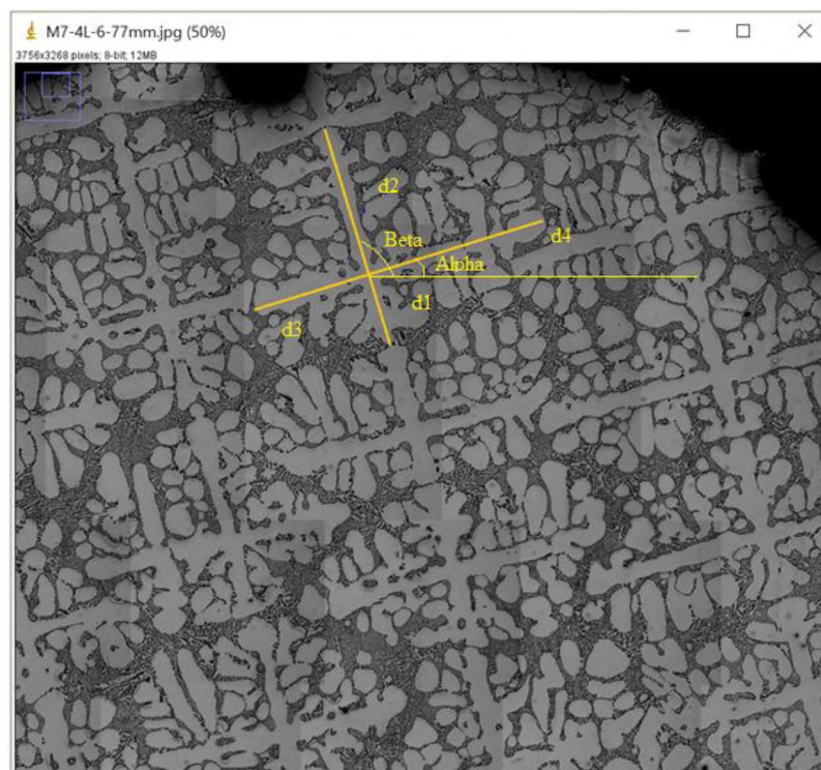
Figure 8. Image of a MICAST sample showing side arm d_1 , d_2 , d_3 , and d_4 location in a dendrite along with angle alpha and beta.
