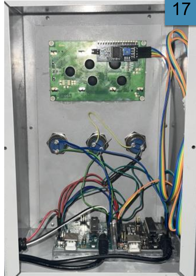
Components box – screen, microcontrollers, buttons, power supplies
