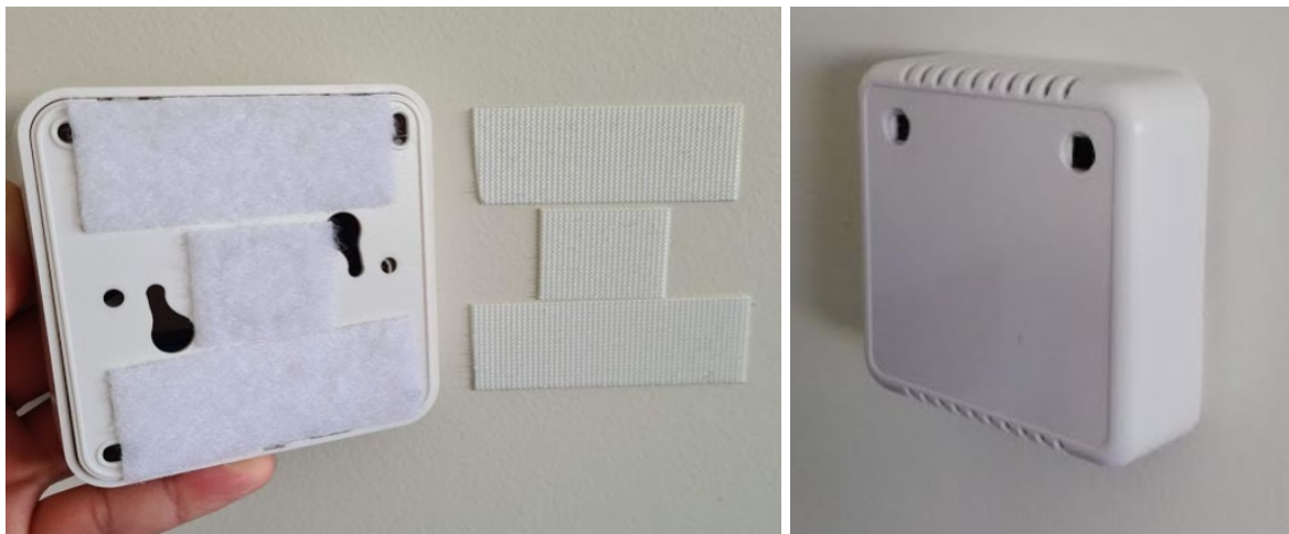
Figure 3. A Bluetooth Low Energy receiver attached to the wall using adhesive tape.
