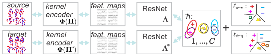
Figure 4.4: Our pipeline: combining the 3D body skeleton encoding and the supervised domain adaptation. Unlike [Koniusz et al., 2017], we utilize two classifiers (one per network stream) and perform alignment between the classes that are shared between the source and target datasets.
