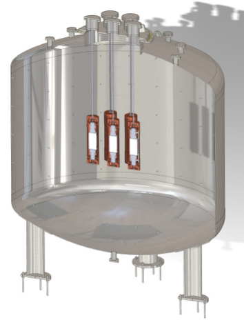
Figure 1: A rendering of the SABRE South detector. The central NaI:Tl detectors are surrounded by a vessel filled with liquid scintillator, while the vessel itself will be surrounded by low-radioactivity passive shielding (not shown).
