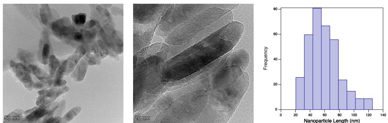
Figure 1. TEM images of the synthesized rutile TiO 2 nanorods, and a histogram showing the distribution of nanoparticle lengths with an average length of 60 \pm 23 nm averaged over 352 measurements.
