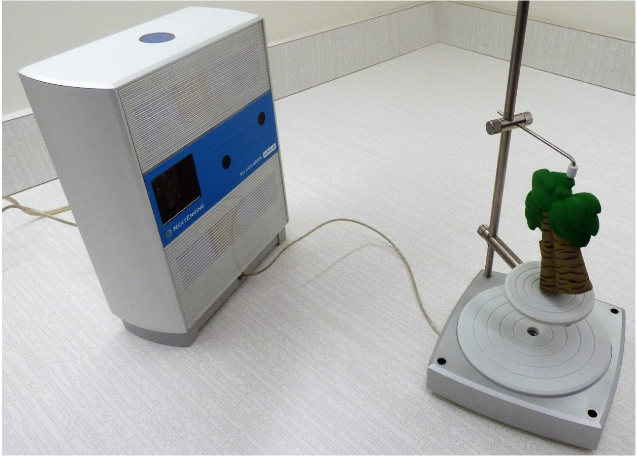
Figure 1.2 The NextEngine 3D Scanner Ultra HD, with integrated turntable. Image credit: NextEngine, inc.
