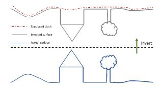
Figure 2. Overview of the Cloth Simulation Filter (CSF). Adapted from Zhang et al. 2016 [18].
