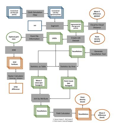
**Figure 3.** Workflow for tessellation comparative analysis using Quanergy M8, Velodyne HDL-32E, and North Carolina Quality Level 2 (QL2) LiDAR data; grey boxes indicate tools and operations, green squares indicate intermediate outputs from the different operations, dark blue boxes represent inputs including the constrained point clouds, and orange objects indicate final products, with squares indicating spatial data and ovals representing metrics.
