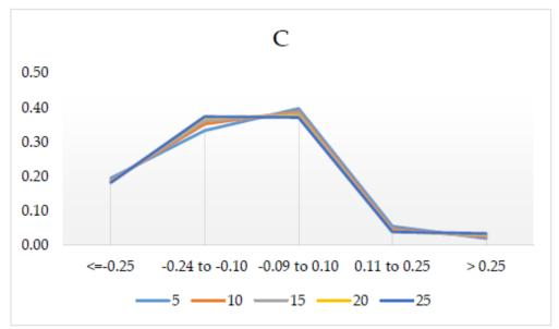
**Figure 6.** The percentage of area (*Y*-axis) for elevation difference (in meters) (*x*-axis) for each tessellation (5 m<sup>2</sup> through 25 m<sup>2</sup>) for (**A**) comparison between the Quanergy and Velodyne sensors; (**B**) comparison of Velodyne with the QL2 data, and (**C**) comparison of Quanergy with the QL2 data.
