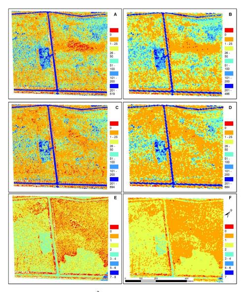
**Figure 4.** Ground point density (points/m<sup>2</sup>) of two LiDAR UAS sensors, the Quanergy M8 and Velodyne HDL-32E, and North Carolina Quality Level 2 (QL2) LiDAR data: (**A**) Quanergy at 5 m<sup>2</sup> tessellation, (**B**) Quanergy at 25 m<sup>2</sup> tessellation, (**C**) Velodyne at 5 m<sup>2</sup> tessellation, (**D**) Velodyne at 25 m<sup>2</sup> tessellation, (**E**) QL2 at 5 m<sup>2</sup> tessellation, and (**F**) QL2 at 25 m<sup>2</sup> tessellation.
