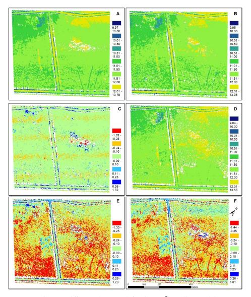
**Figure 5.** Mean elevation difference (in meters) for the 5 m<sup>2</sup> tessellation: (**A**) Quanergy M8, (**B**) Velodyne HDL-32E, (**C**) difference between the two UAS LiDAR sensors (Velodyne – Quanergy), (**D**) North Carolina Quality Level 2 (QL2) LiDAR elevation, (**E**) difference between Velodyne and QL2, and (**F**) difference between Quanergy and QL2.
