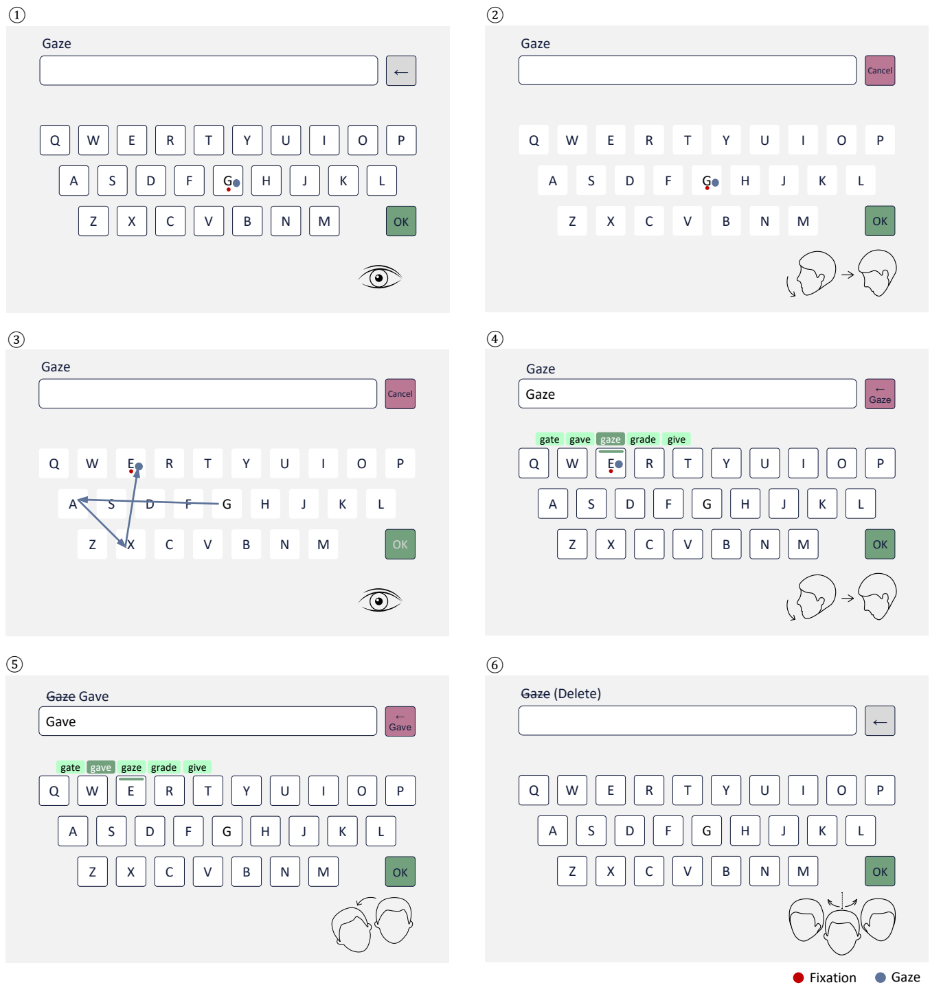
Figure 1: The HGaze Typing interface. The text to be entered is shown above the text box (“gaze”). The word can be typed by completing the following actions: (1) Fixate on the first letter of the desired word. The red dot on the key indicates a fixation. (2) Select the key with a nod. (3) Glance through the intermediate letters. The corresponding gaze path is used to compute the candidate words. (4) Fixate on the last letter and selected by a nod. The most probable word is typed, and a candidate list with five words is shown above the key. (5) If desired, change the typed word with a head tilt (left or right). (6) Use a shaking gesture to delete a typed word (a shake can also be used to cancel a gaze path).
