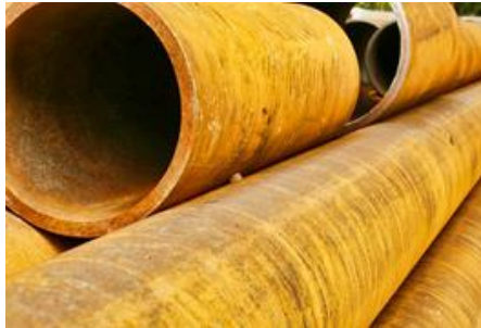
Figure 1.3: Pipelines already covered with rust [37]
