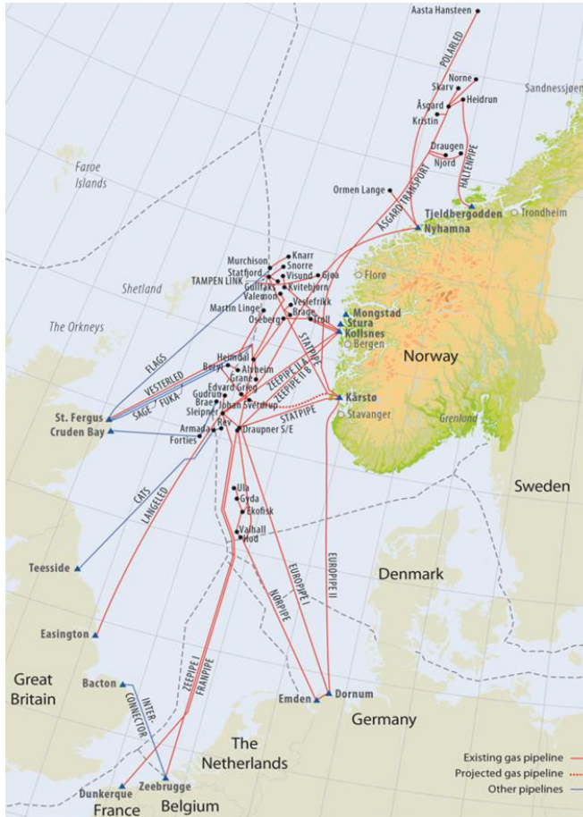
Figure 1.1: Network of pipelines in the Norwegian Continental Shelf, showing Europipe I, Europipe II and others [30]
