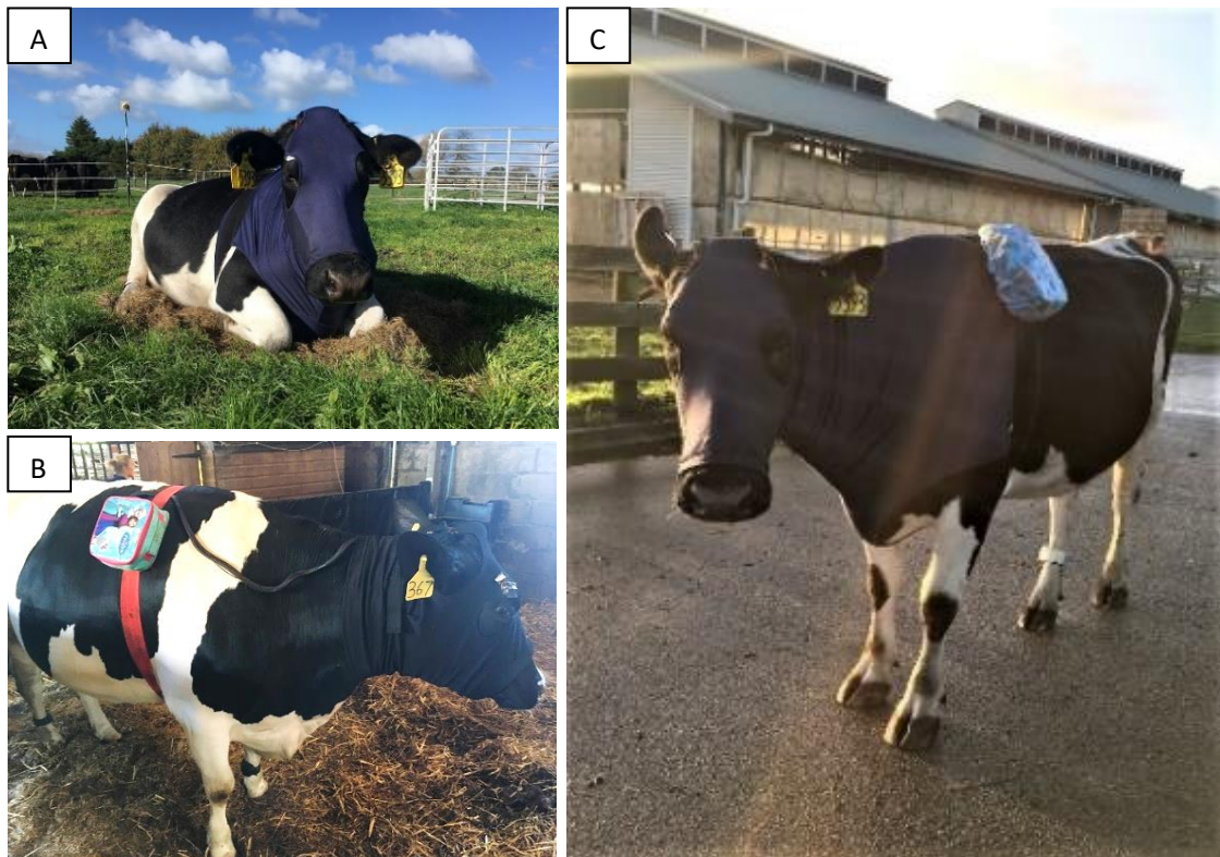
Figure 7. [A] Cow in New Zealand wearing a modified Lycra hood [B] A cow in Scotland wearing a modified 'summer' hood with electrode wires bundled along the neck to the device housing attached to the girth, [C] A cow in New Zealand wearing the full hood and with a waterproof plastic cover over the device housing pouch.
