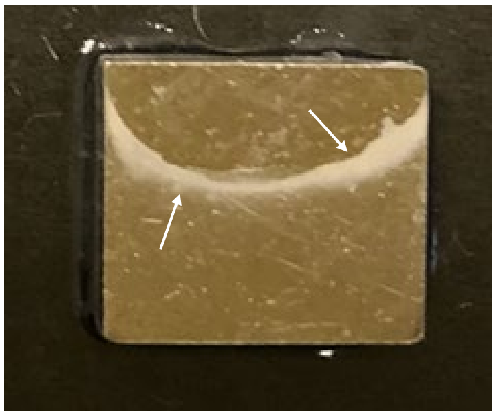
Figure 5. 1 Biomass on a SS coupon formed by P5 after 24 h of incubation. The white arrow indicates the visible biofilm.
