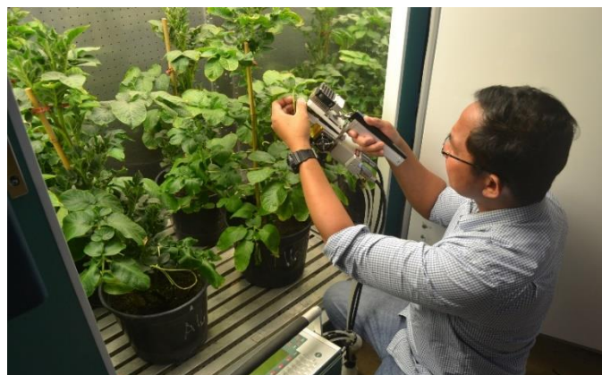
Figure 5.6 Measurement of net photosynthesis ( P_N ), transpiration rate ( E ), and stomatal conductance ( g_s ) using LI-COR portable photosynthesis system in the plant growth chamber.
