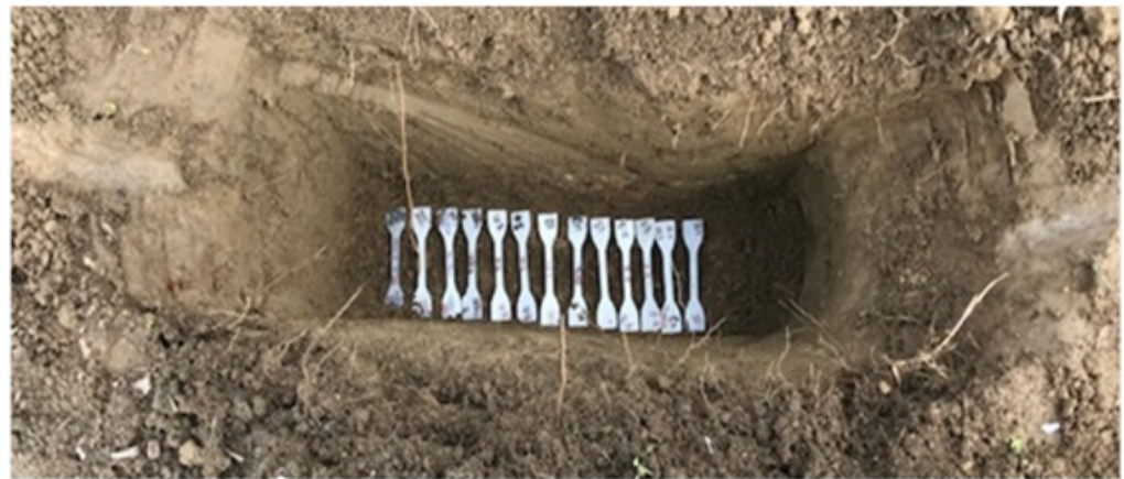
Figure 3. Location and orientation of buried samples for soil degradation.
