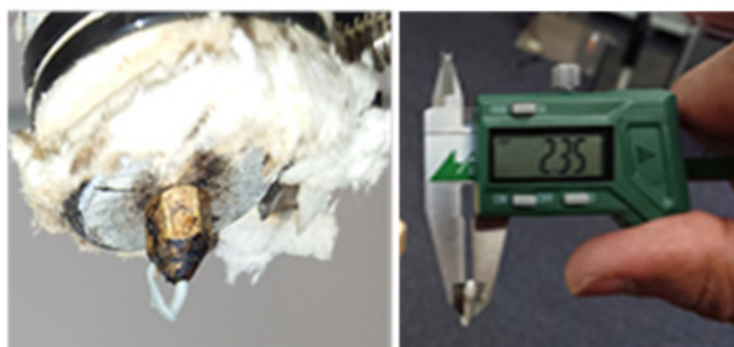
Figure 1. Die swelling in extruded filament from pellet printer.
