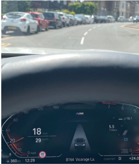
Figure 13: Example of traffic sign recognition error indicating 80mph in a 30mph urban area (Vehicle: BMW).
