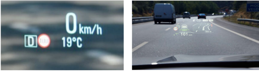
Figure 12: Heads Up Display (HUD) showing Speed Limit Sign Detection. Vauxhall (L) and BMW (R).
