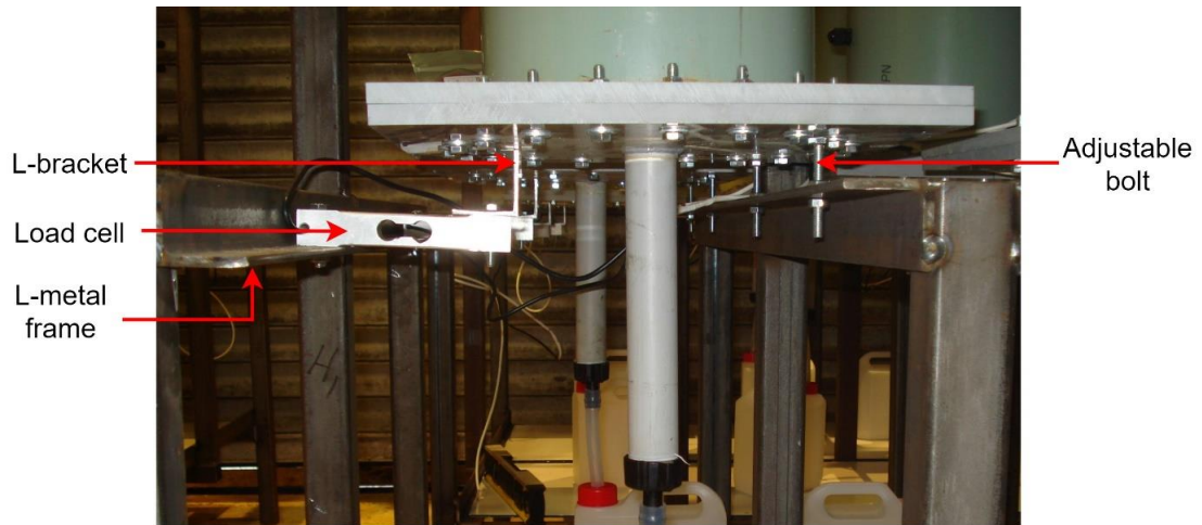
Figure 3.5. The side view of load cell assembly and lysimeter resting position on the load cell.
