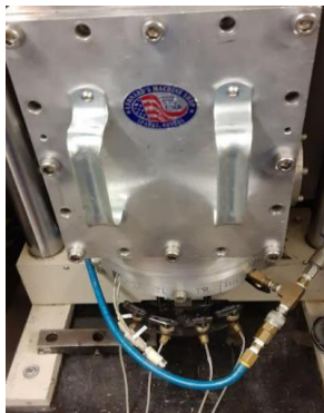
Figure 27. Closed Chamber and Drainage Valves.
