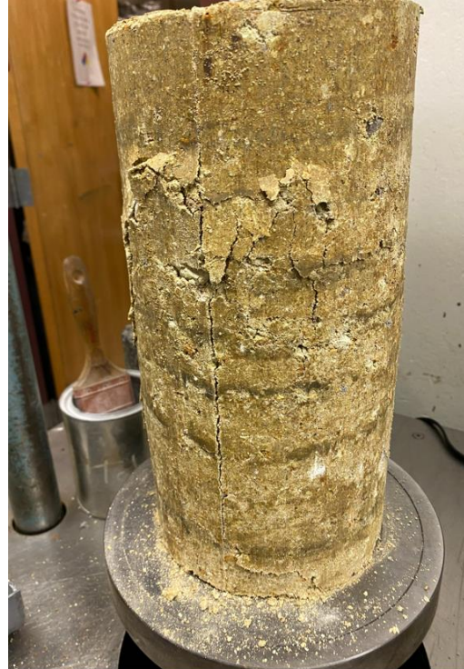
Figure 17. UCS Sample After Testing.
