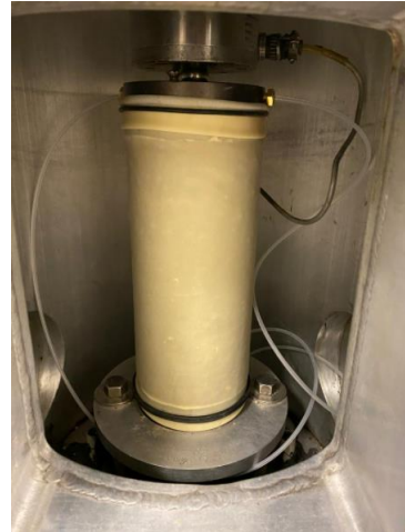
Figure 26. Sealed Sample in Triaxial Chamber.
