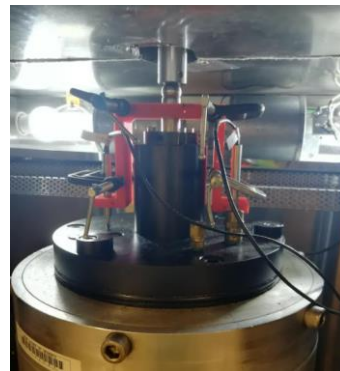
Figure 28. LVDTs Connected Outside the Chamber.
