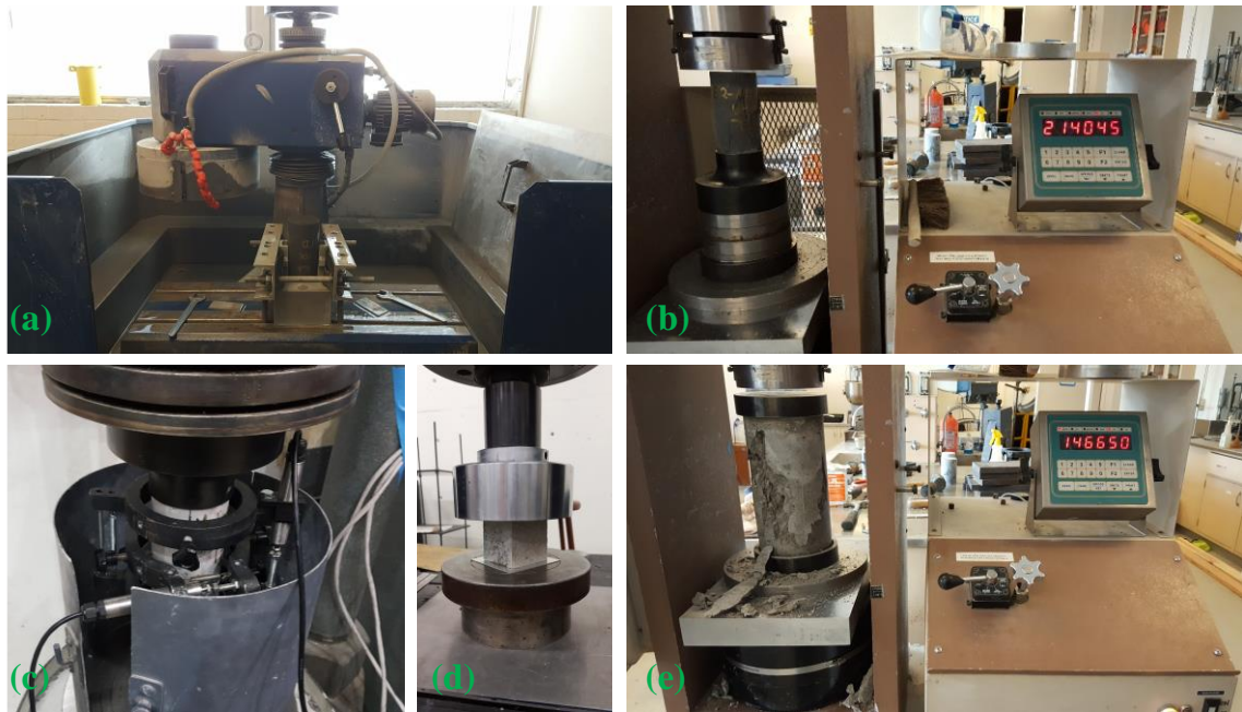
Figure 3-11 (a) Grinding of UHPC and PMMA-PC cylinders; and compression testing of: (b) 7.6 \times 15.2 cm UHPC cylinders, (c) 7.6 \times 15.2 cm PMMA-PC cylinders, (d) 5.1 cm PMMA-PC cubes, and (e) 15.2 \times 30.5 cm conventional concrete cylinders
