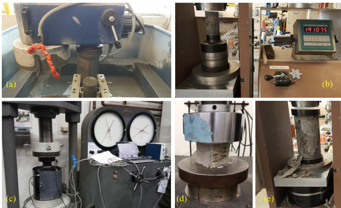
Figure 2-8 (a) Grinding of UHPC and PMMA-PC cylinders, and compression testing of: (b) 3×6 in (7.5×15 cm) UHPC cylinders, (c) 3×6 in (7.5×15 cm) PMMA-PC cylinders, (d) 2-inch (5.1 cm) PMMA-PC cubes, and (e) 6×12 in (15 × 30 cm) NSC cylinders
