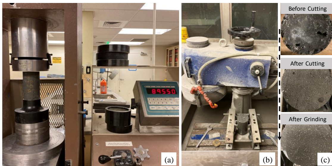
Figure 4-6 Compression testing of NP-UHPC cylinders: (a) test setup; (b) grinding machine for cylinder preparation; and (c) views of typical NP-UHPC cylinder through preparation sequence.
