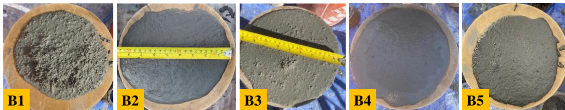
Figure 4-5 Static flow of the fresh NP-UHPC mixes.
