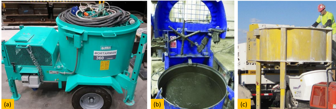
Figure 7-6 Examples of the UHPC mixer types (a) IMER high shear mixer, (b) high shear pan mixer [13], and (c) portable concrete pan mixer [12].
