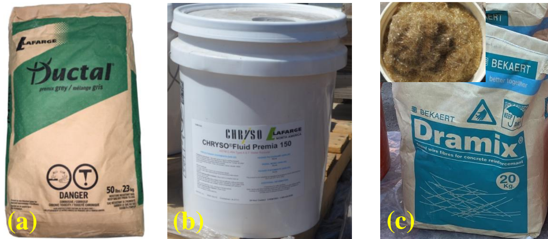
Figure 7-5 Ductal® UHPC components (a) dry premix, (b) superplasticizer, and (c) steel fibers.
