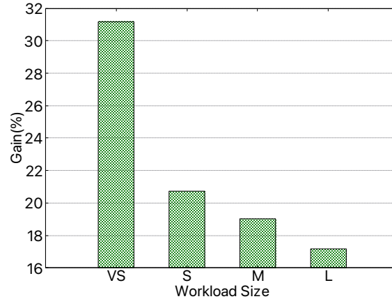
Figure 4.3: Performance comparison between network-aware scheduling using delay-based nodes ranking strategy and nearest node selection-based scheduling strategy for various workload sizes: very small (VS), small (S), medium (M) and large (L) on serverless computing workload .
