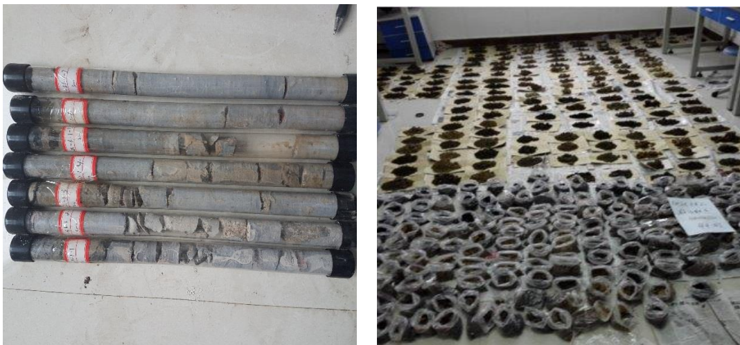
Figure 2.4: Images of the sample collection and initial processing a) the rock samples collected in the cores and (b) pit soil samples were air dried before shipment to the UK (picture credit: Dr H. L. Buss).
