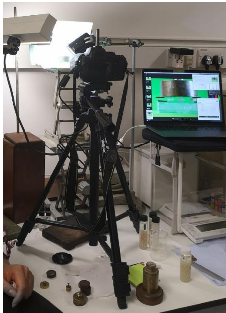
Figure 5.5. Set-up for compression test pictures.
