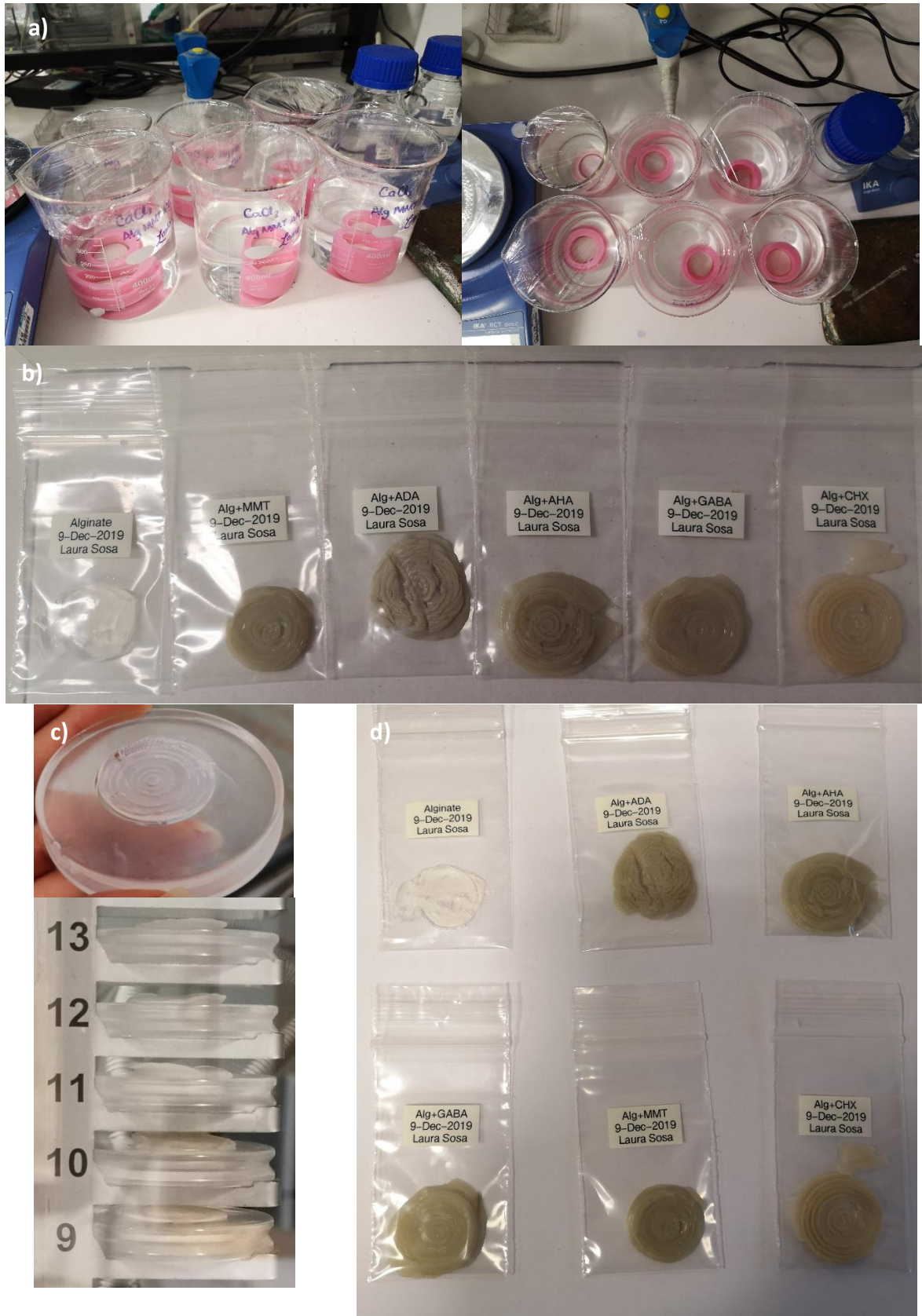
Figure 5.8. a) Silicon moulds for making the hydrogel discs, b) all hydrogel samples after XRD characterization, c) samples in holder for XRD and d) all hydrogel samples after being left outside wet environment for 1.5 months.
