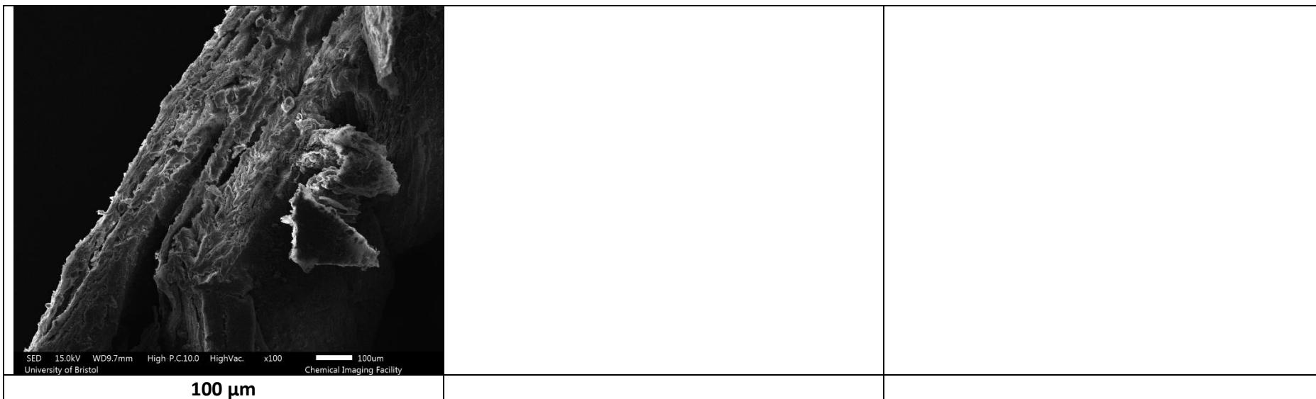
Figure 8.12. SEM images of Alginate (Alg) + modified clay (MMT CHX) sample – Cross section.
