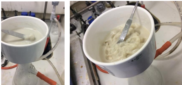
Figure 2.7. Sample of MMT+GABA 3x HCl being filtered for cleaning purposes.
