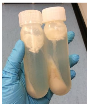
Figure 2.6. Sample of MMT+ADA 24h after being centrifuged for cleaning purposes.
