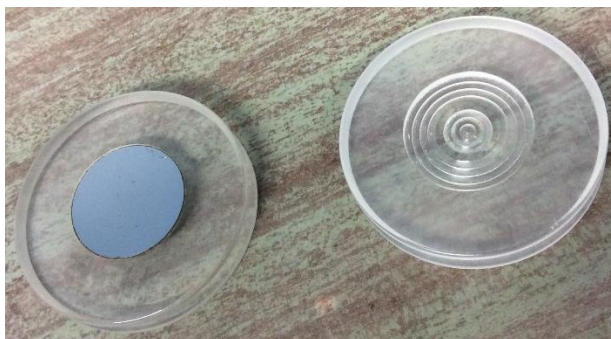
Figure 2.4. On the left, sample holder made of silicon used for smaller amount of sample and on the right, sample holder made of plastic for larger amount of powder.
