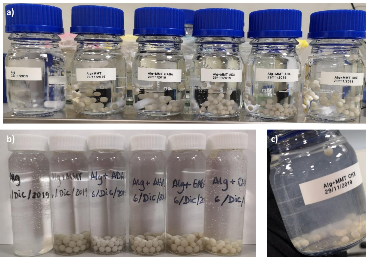
Figure 5.7. a) Six samples during preparation, b) six samples after 7 days, c) Alg + MMT 1.2 CHX beads after 7 days before rinsing.
