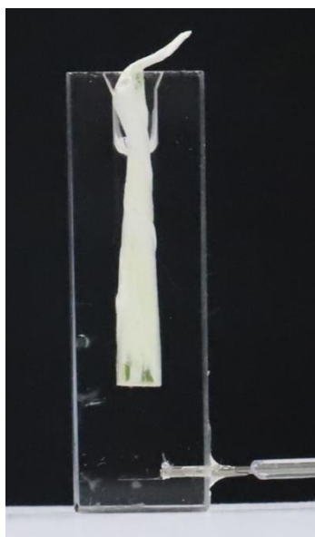
Figure 4.3-7: Dampened oscillation device. An optical cuvette was used as the oscillation-column and a small hole was drilled right at the bottom which was fitted with a small metal tube ( \varnothing = 0.7 mm) that was connected to a syringe mounted to a syringe pump. From there, hydrogen-peroxide solution was fed into the cuvette system. To reduce the oscillation-length, a PTFE-membrane was wrapped around a yellow Eppendorf-pipette tip (200 \mu L) and inserted into the cuvette, eventually leaving a 8 mm gap between the bottom and the membrane.
