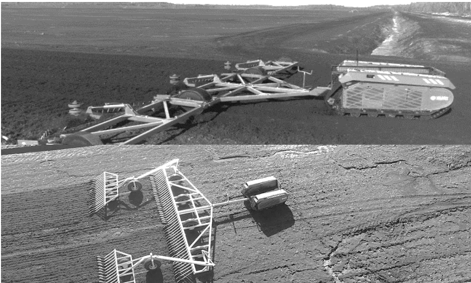
Figure 4. (up) The passive miller and (down) the harrower used in the experiment. For both implements the drawbar pull and drawbar power were determined.
