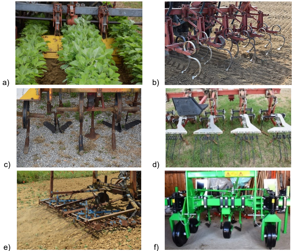
Figure 1. Equipment utilized in the experiments: a) T2 18 – ‘Breviglieri’ equipment, M21-2 model; b) T5 18 and T2 19 – ‘Gaspardo’ equipment, HL-6R model; c) T4 18 – ‘Spapperi’ equipment without crop guard between horizontal knives; d) T3 18 – ‘Badalini’ equipment. Due to the amaranth growth stage, flex tine harrows were not used; e) T3 19 and T5 19 – Equipment without brand name (handcrafted design); f) T4 19 and T5 19 – ‘Sfoggia’ equipment, Kress model.
